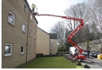
The CMC 19N Arbor Pro (now available with safer, non-slip outrigger pads and a new arborist saw holder) has been built for one of the roughest industries on this planet - the tree industry.
