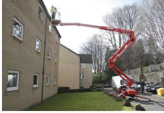
CMC S19 N version "N" is the most compact spider lift access platform available in this size range with the shortest stabilising width area at less than 3 metres!
