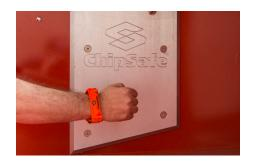
A reset sensor box is located on the outer sides of the infeed chute. By simply swiping the strap on their wrist across the reset sensor box, the operator is able to reactivate the feed mechanism and continue the chipping operation with little or no disruption in productivity.
