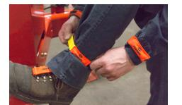
When preparing to use a brush chipper equipped with the ChipSafe device, operators must wear ChipSafe straps on their wrists AND ChipSafe straps on their ankles or ChipSafe bootlace straps on their boots.
