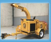
The Rayco RC1220G features a powerful feed system using a planetary drive motor to power the feed wheel for years of dependable service with very little maintenance. To reduce trimming, the throat opening is 20" wide all the way through to the drum, eliminating neck-downs behind the feed wheel.
