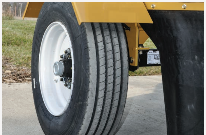
Torflex Suspension Axle with (2) 235-75R-17.5H 6000 lb tires
