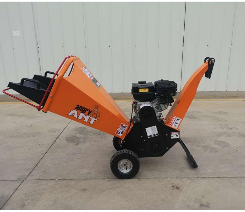
Powered by a 6.5hp Petrol engine, the Angry Ant wood chipper will easily handle brushy material,wood off-cuts and other vegetation material up to 2 inches. Due to its compact design, weighing in at 100 kg the Angry Ant 2-inch wood chipper is light and easy to move around. It will enter confined spaces without difficulty.
