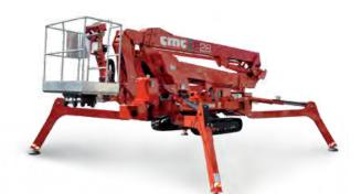
Platform with two articulated telescopic booms plus jib. A concentrate of power and technology ready to amaze. With four stabilization areas, two work areas and stabilizers to "overpass", it is able to work on any terrain and reach even the most inaccessible places. Twenty-eight meters maximum working height, 14 m outreach and 6.7 m under floor level make it an unparalleled platform.
