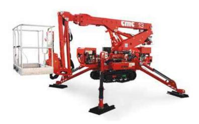
Compact, light and versatile, S13F is the perfect solution in the most difficult conditions and in the most narrow spaces. Fully hydraulic, with two working areas and a telescopic boom with 2 extensions plus jib (90°) it is a platform simple to use, intuitive and fast. Thanks to its small size, it passes through a standard door and enters in the elevators.
