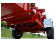
Channel Frame Full length channel chassis with cross bracing, this increases structural strength while maintaining low unit weight.
